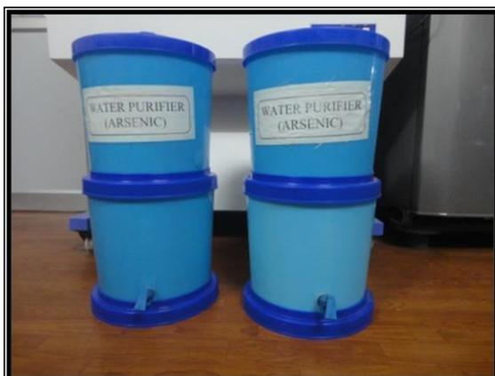
Water filtration system for removal of fluoride and arsenic (Domestic model – 15 L capacity) has been developed which has arsenic removal efficiency of 87 % and Fluoride removal efficiency of 92 %. The Cost of the model is Rs. 1000.00. The model has been installed at Government school, Mavinamatti, Shahapur, Yadgir (Dist.) in collaboration with IIT, Chennai for removal of arsenic from drinking water.
